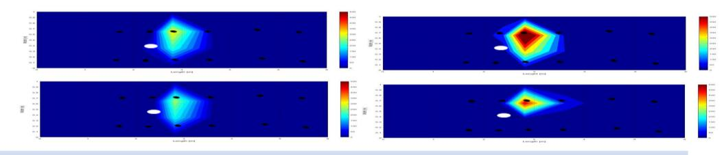
After the injection of NANOFER STAR, an increase in PCE degradation could be observed. Production of degradation products Cl<sup>-</sup>, ethene and ethane were also observed 1 week after the injection (graph below). Even after 90 days of the injection, the PCE degradation is still in progress. As a preliminary result, the STAR particles had degraded m = 190.3 g of PCE after 90 days, based on the produced mass of Cl<sup>-</sup> in the outlet.
