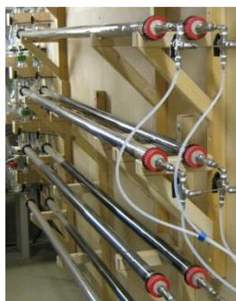
Experimental setup for reactivity studies in columns © VEGAS/USTUTT
