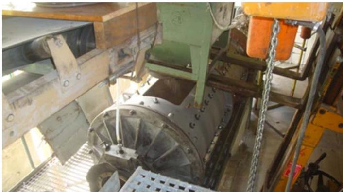
**Figure 8: Filling operation of the ball mill**
