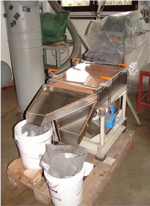
Figure 9: Sieving of milled particles after dry milling, Dreßler type (400 x 600 mm)
