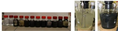
Fig. 2: Left – Reagent bottles for kinetic batch tests; Right – reactors
