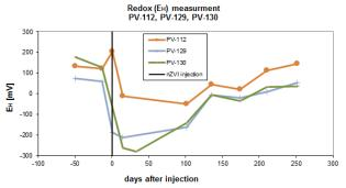
Figure 16. Redox potential after NANOFER STAR injection
