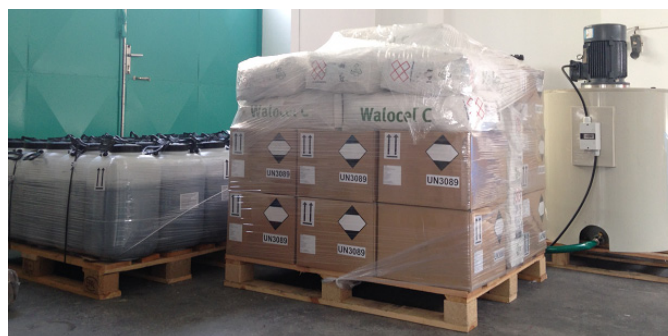
Figure 1. Photograph showing nanoremediation products and equipment prior to departure to the NanoRem Spolchemie I site. On the left are plastic barrels containing NANO FER 25S slurry, in the middle are boxes of NANO FER STAR, together with bags of the stabiliser carboxymethyl cellulose, and on the right is the dispersing unit (© NANO IRON s.r.o.)
